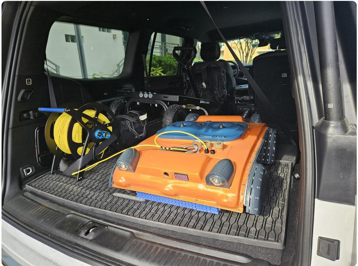
Nakai's robots are autonomous cleaning vehicles that remove biofouling — a buildup of algae, vegetation, and animal life — on ships, helping them run more efficiently. The Nakai robots include 1,500 different components, and 300 of them are 3D printed for end-use on the Fuse Series and Form Series. Their SLS components are coated in ceramic to keep them waterproof.
