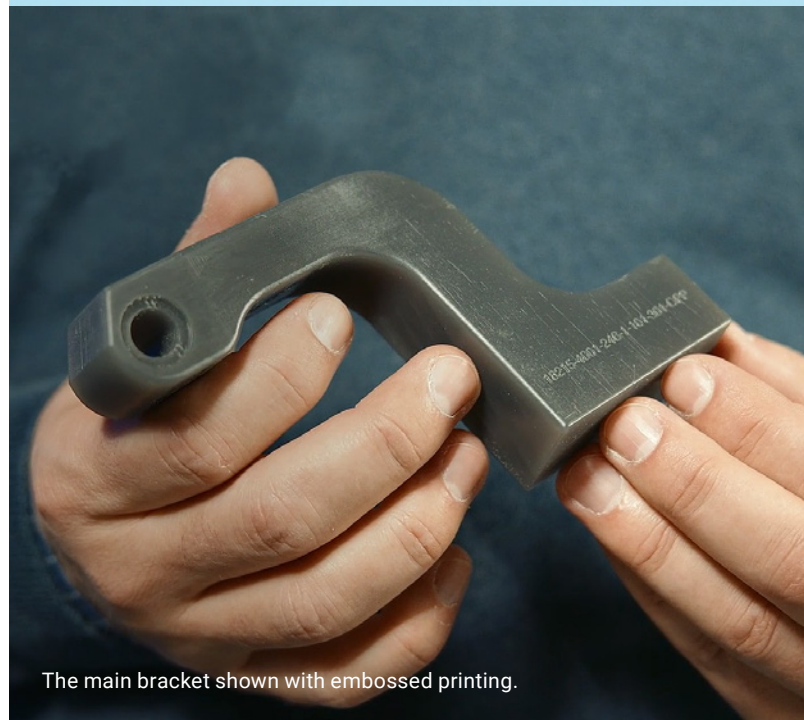
The 3D printed main bracket made with Loctite® 3D 3172 resin in the Origin One.
