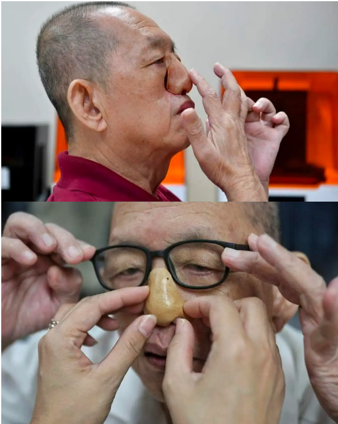
Form, fit, and function testing of the 3D printed nose prosthetic on Mr. Lian.
