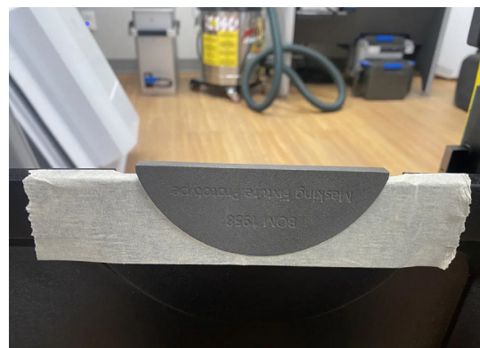
In the first step, tape covers a large section of the part. In the second, the 3D printed part acts as a stencil around which a technician will cut the rest of the tape away, ensuring that the copper-coated part remains free of paint, while the rest of the surface is painted black.
