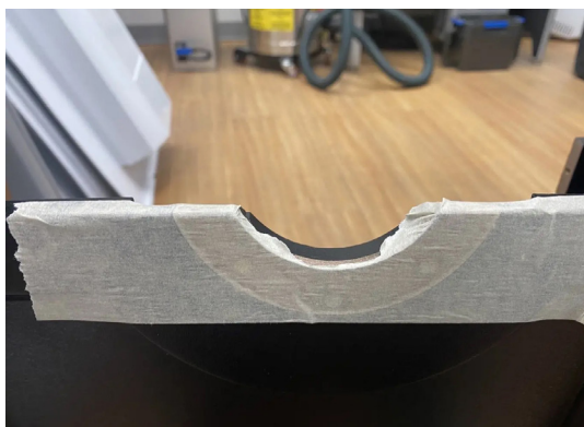
In the first step, tape covers a large section of the part. In the second, the 3D printed part acts as a stencil around which a technician will cut the rest of the tape away, ensuring that the copper-coated part remains free of paint, while the rest of the surface is painted black.
